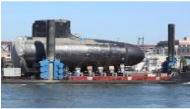
USS Colorado bow hull section en route from Newport News via NY East River to Electric Boat shipyard in Groton (Photo courtesy of usscoloradocommittee.org/ )
